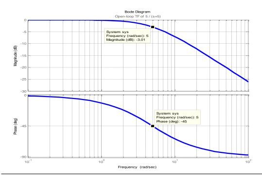
Bode diagram of open-loop transfer function is
